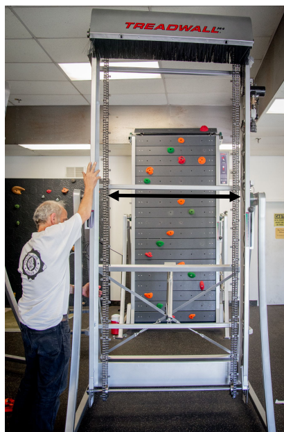
Check chains area synchronized: tab are level with each other on both sides. Use the spacer bar as a guide.
