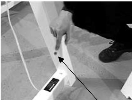
**Many of the nuts, bolts and washers are shipped attached to the appropriate parts.** The bolts, nuts, and washers are in the proper orientation and order and should be kept the same way during assembly.
