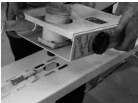
← □ **Attach the control panel to the channel.** Remove the four bolts that hold the pump to the control panel. Also remove the nut and washers from the "fifth bolt" that is right below the pump and take the large washer off the pump shaft. Place the control panel on the channel as shown and use the four mounting bolts to attach through the slots. Each bolt must have a flat washer to slide against the channel and a lock washer to hold it tight. See the tightening instructions below.
